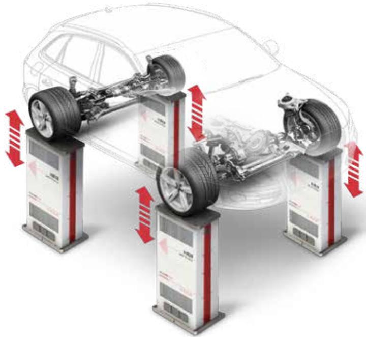
Damper Test System HUD020 with 4 synchronized machines
