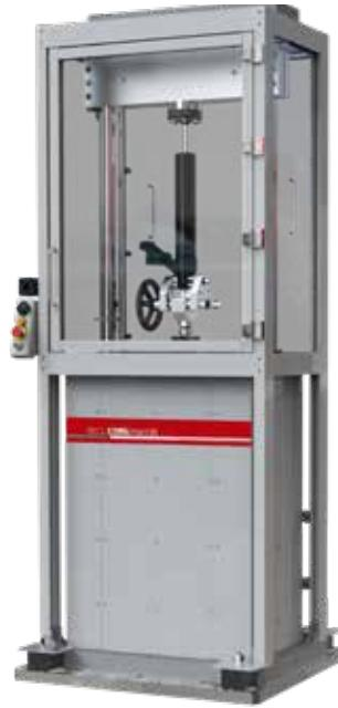
High dynamic system for durability testing
