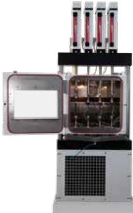
Creep testing machine with up 5 axes
