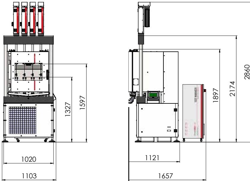
Creep testing machines with 4 axes - Dimensions
