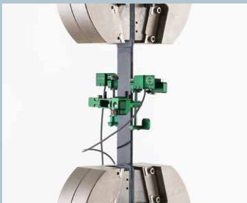
Model 3442AVG extensometer 3442-050M-025M-ST
