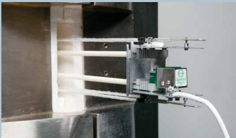
Self-supporting Model 3448 with clamshell-type materials testing furnace
