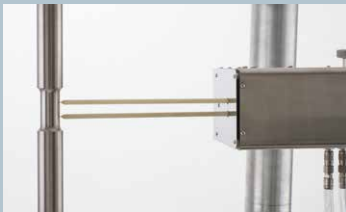
Model 7650 extensometer with 12.5 mm gauge length
