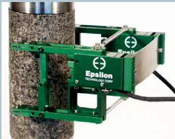
Model 3542RA1 extensometer with 50 mm gauge length
