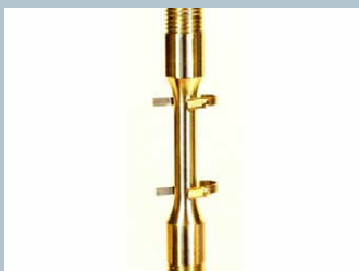
Laser extensometer high temperature clip-on reflectors
