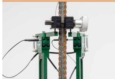
Model 3567 specimen attachment collar with extensometer installed
